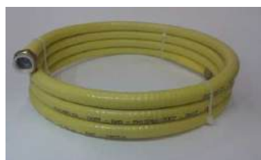
FLEXIBLE HOSE CSST DN12, IN STAINLESS STEEL AISI316L THICKNESS 0,30 mm. COVERED WITH YELLOW PE SHEATH THICKNESS 0,5 mm. ASSEMBLED WITH TWO 1/2" NUTS COMPLETE WITH GASKETS PRODUCT STANDARDS UNI EN 15266 AND UNI 7129 INSTALLATION STANDARDS
