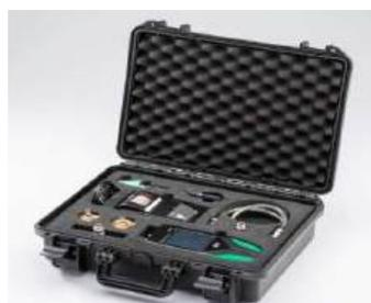
KIT PER PROVA TENUTA IMPIANTI GAS COMPOSTO DA: VALIGETTA STAGNA IP67, STAMPANTE, ALIMENTATORE + CAVO USB, BATTERIA AL LITIO, RACCORDI FILETTATI, RACCORDO INNESTO RAPIDO DA 1/4", RACCORDO A 3 VIE, TUBO DI COLLEGAMENTO E CONO IN GOMMA
